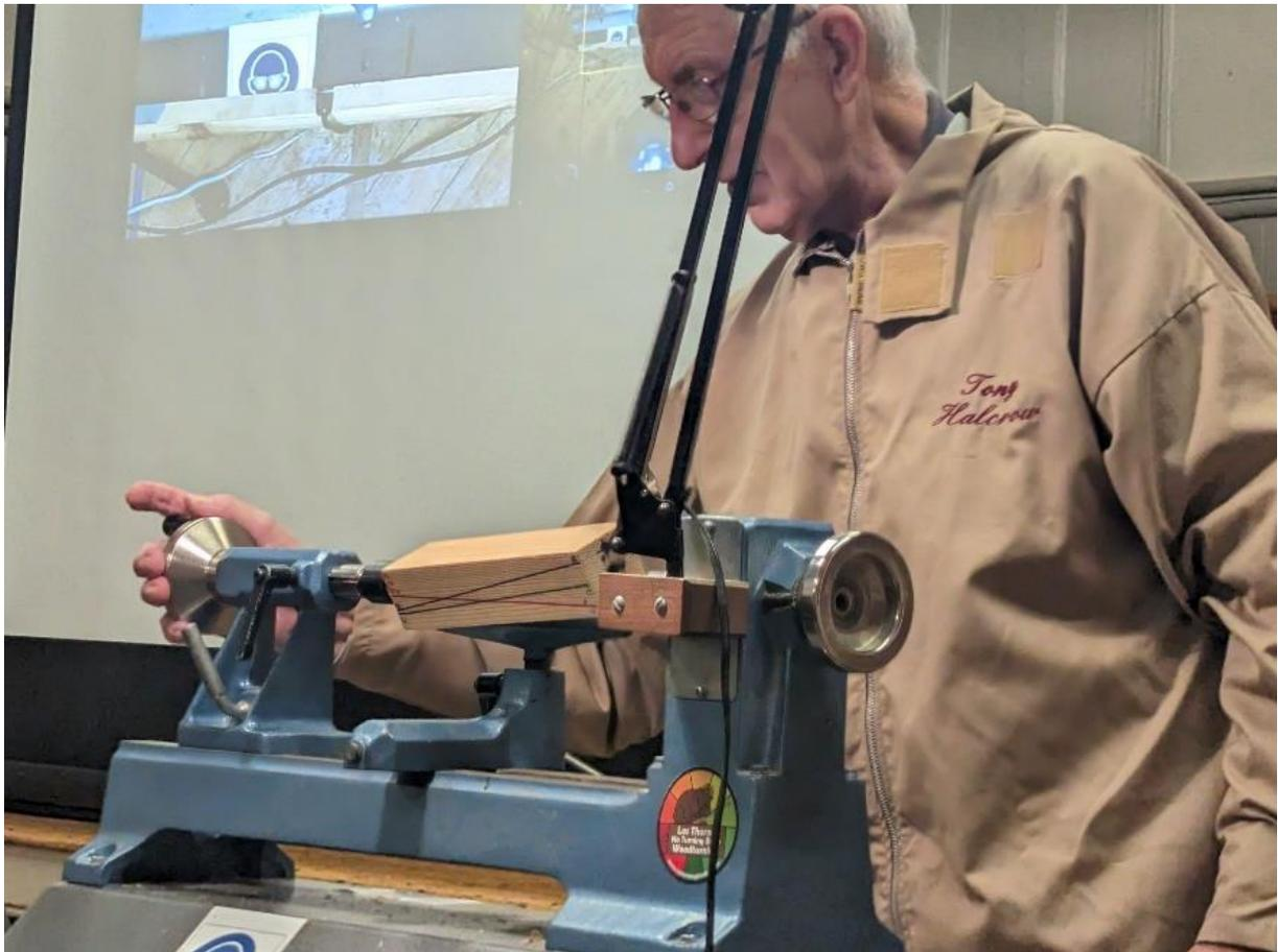
This was achieved by working on three axes, starting with the head and shaping each section before moving on the next. Tony explained that care is required where the axes intersect as it can be easy to remove too much material and cut through the piece entirely.
