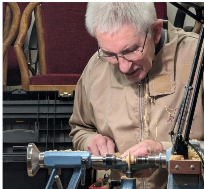
The item was again turned from a single piece of wood, but Tony elaborated on alternative approaches to work-holding which made the task a little easier and was amenable to incorporating additional decoration/finials on each end perpendicular to the ring. This was evidenced by a piece he had prepared earlier, featuring a tiny goblet with captive ring on each pole of the “planet”.
